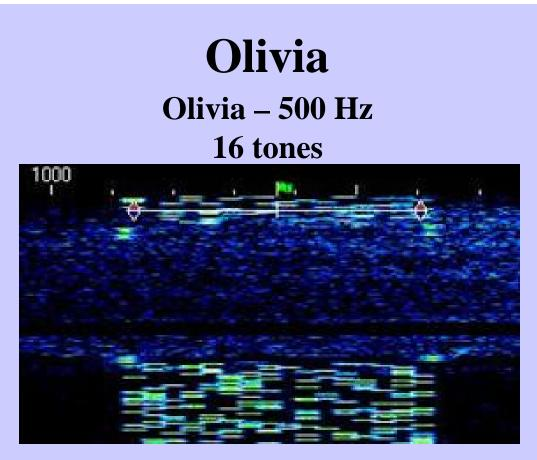
Our standard is 16/500 but other common Olivia operations are transmitted in 250, 500 and 1000Hz bandwidths. Tuning and sound card calibration are critical on this mode, but Olivia is capable of maintaining near 100% copy under extremely adverse conditions.
