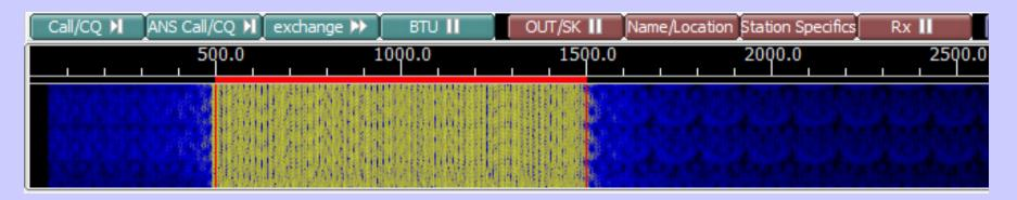
MT63 1k long was chosen for portable, mobile and fixed station operations on HF USB under moderate to good conditions. It is our primary mode for detailed situation reports and database transmissions on HF for the following reasons:
