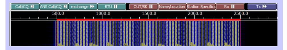
MT63 2k long was chosen for local portable, mobile and fixed station operations on FM channels (repeater or simplex). It is extremely well suited for detailed situation reports and database transmissions for the following reasons:
