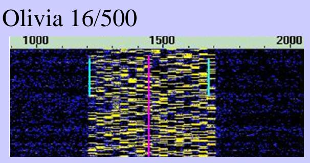
Olivia 16 tones, 500 Hz mode was chosen for use in formal short message handling. Although the mode is relatively slow (about writing speed), it is very accurate, even under extremely poor conditions.
