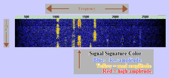
The digital waterfall is a visual representation of time, frequency and amplitude.
