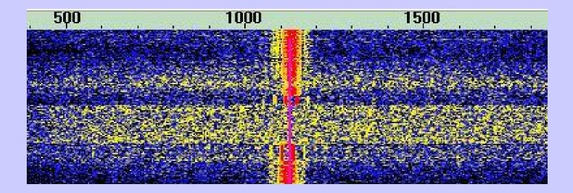
You will notice the slight shift from the two stations signals. Most PSK31/63 software will automatically track slight shifts with the AFC (Automatic Frequency Control) setting. NBEMS/FLDIGI is one of the best in this respect. But AFC is not available with Olivia and MT63, so sound card calibration can be critical.
